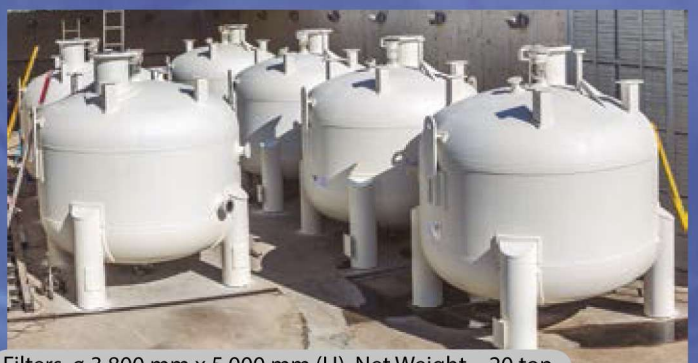
Filters, \phi 3,800 mm x 5,000 mm (H). Net Weight – 20 ton.
