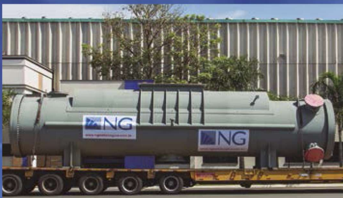
Condensing System, \phi 2,380 mm x 12,800 mm. Net Weight – 101 ton.
