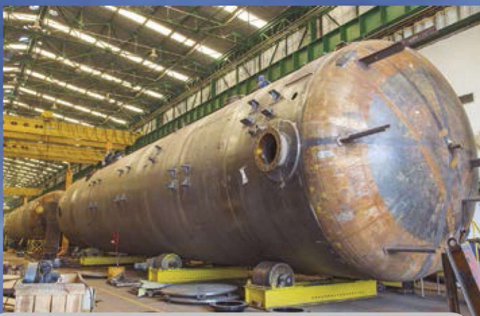
Deaerating Towers, \phi 4,500 mm x 19,900 mm. Net Weight – 90 ton.
