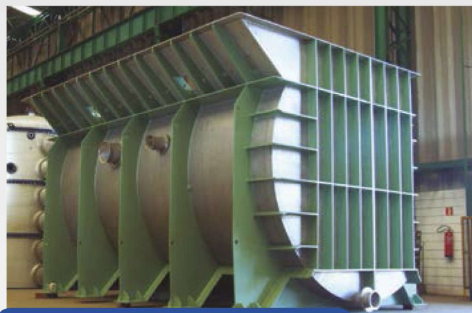
Pulper Tank, 2,800 mm x 6,800 mm x 3,800 mm.
