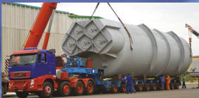
Sulphur Furnace, \phi 5,200 mm x 19,800 mm. Net Weight – 76 ton.
