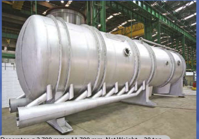
Deaerator, \phi 2,700 mm x 11,700 mm. Net Weight – 20 ton.
