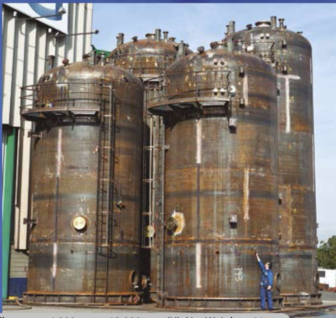
Floaters, \phi 4,800 mm x 13,000 mm (H). Net Weight – 44 ton.
