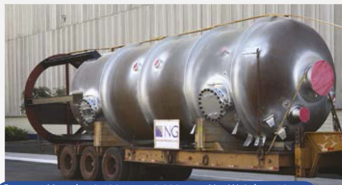
Pressure Vessel, \phi 2,400 mm x 8,000 mm. Net Weight – 10 ton.
