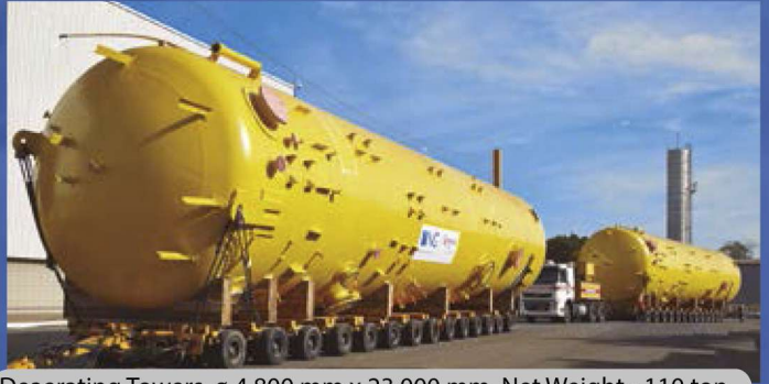
Deaerating Towers, \phi 4,800 mm x 23,000 mm. Net Weight - 110 ton.
