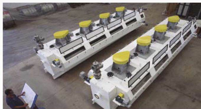
Floaters, \phi 11,000 mm x 2,900 mm x 2,000 mm. Net Weight – 7 ton.
