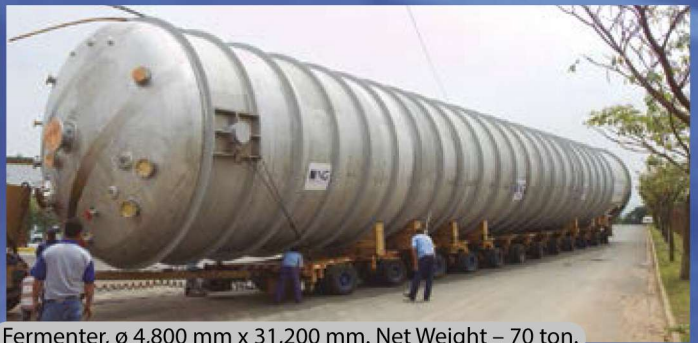
Fermenter, \phi 4,800 mm x 31,200 mm. Net Weight – 70 ton.
