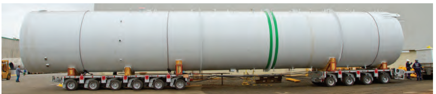
Torre Desaeradora/ Deairing Column ("U" Stamp) co/l - 19.900 mm LT/LT Ø 4.500 mm
