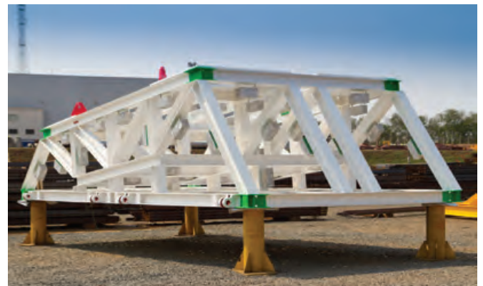
Plem/Plem co/l - 9.000 mm la/w - 6.944 mm a/h - 2.420 mm p/we - 17.551 kg
