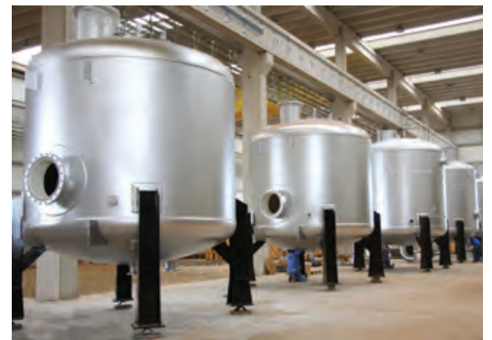
Filtros/Filters Ø - 3.800 x 3.200 mm LT/LT
